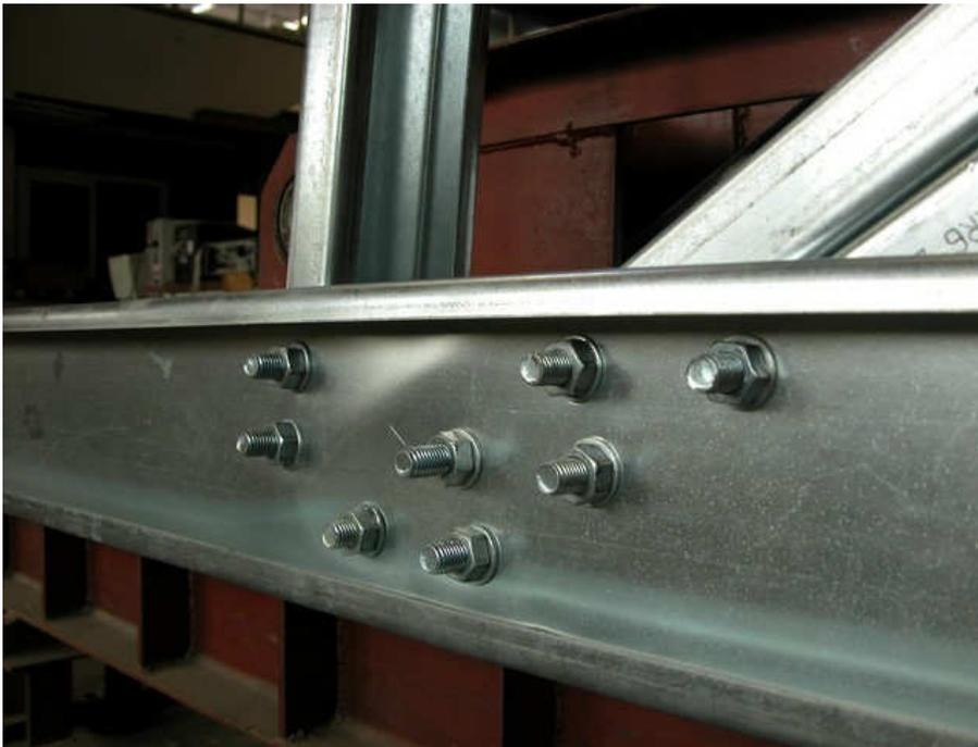
failure in the lower chord joint nearest to the support; interaction of shear and tension
