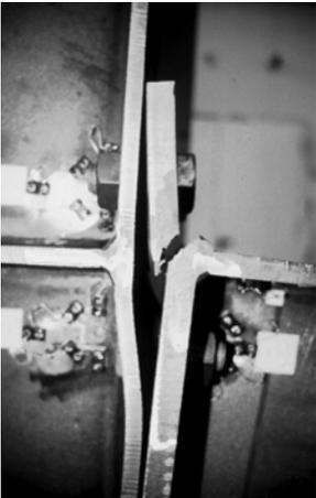
Fig. 13 Failure by rupture in the end-plate, test Z2
