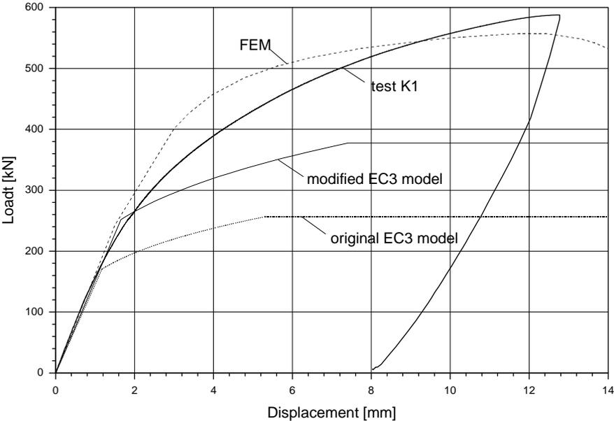
Fig. 9 Load-displacement diagram for test K1 with bolts M24
