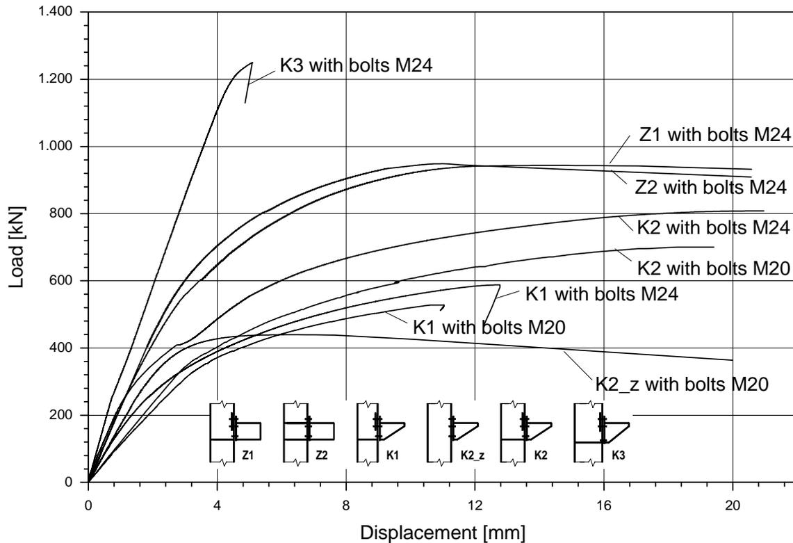
Fig. 7 Summary of load-displacement diagrams
