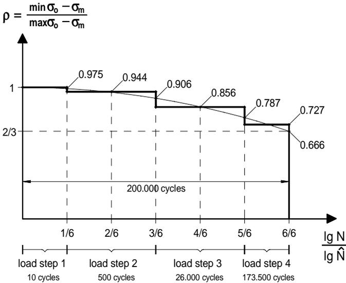
Fig. 10 Load spectrum curve and its step-like approximation
