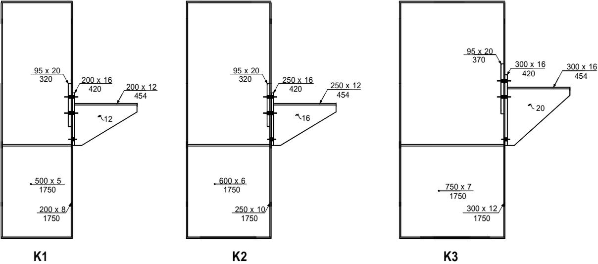
Fig. 3 The test specimens
