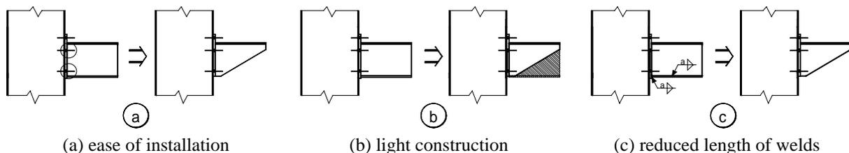
Fig. 1 Crane bracket design advantages
