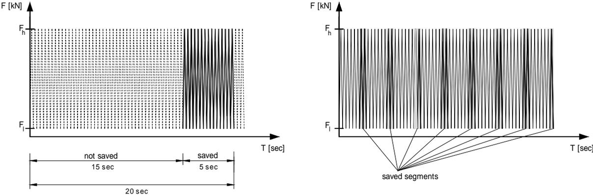
Fig. 11 Principle of the saving the measured data
