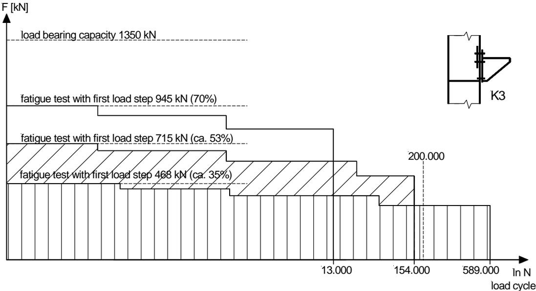
Fig. 12 Test specimen K3 under repeated loading with different load spectra
