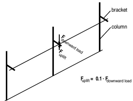
Fig. 6 Illustration of uplift load
