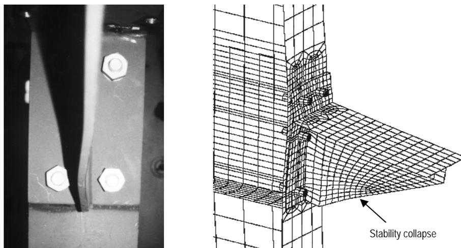
Fig. 8 Bracket web after stability failure in test specimen K1 and the FE model under ultimate load
