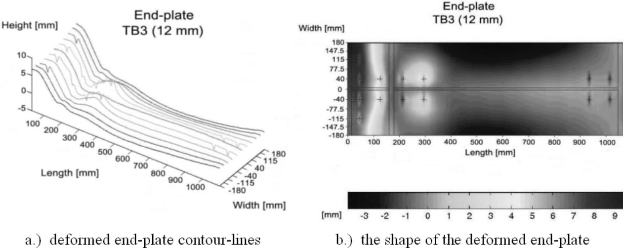
Fig. 8. Evaluated results of the measurement on the deformed end-plate of specimen TB3
