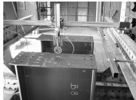
Fig. 4: Measuring the plastic deformation of the end-plate
