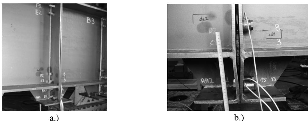
*Fig. 5.* Specimen TB3 - arrangement and failure mode
