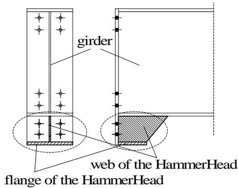
Fig. 1. The HammerHead arrangement
