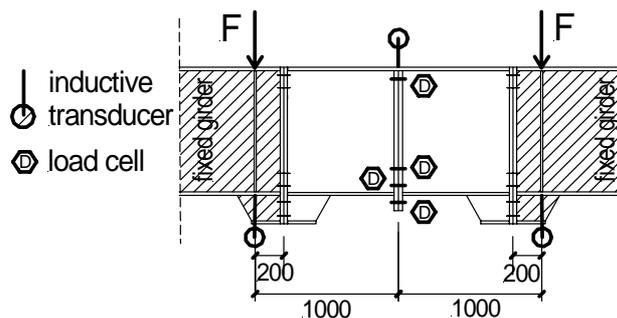
Fig. 3. Locations of transducers and load cells
