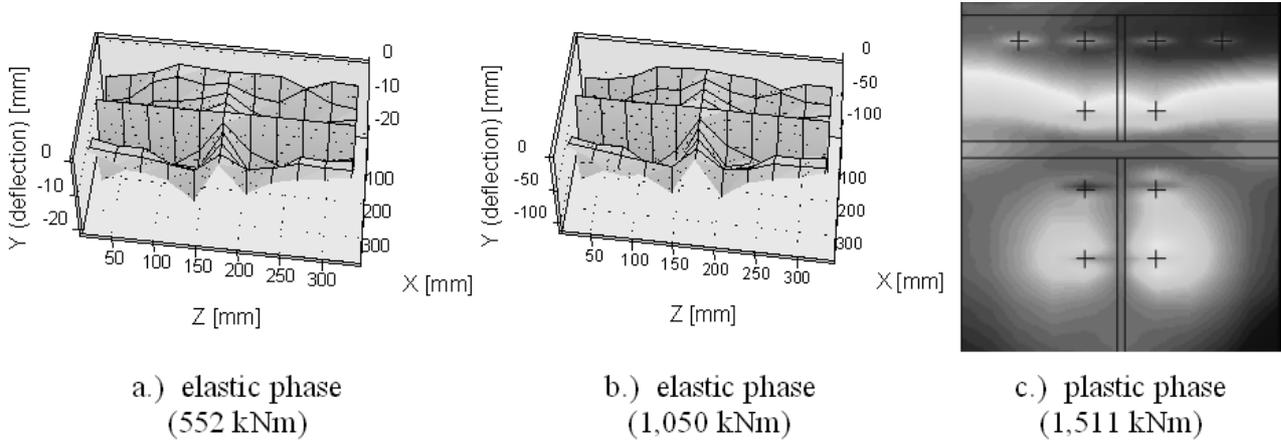
Fig. 7. The end-plate deformations in the elastic and the plastic phases of the specimen TB3
