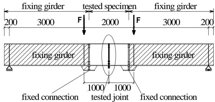
Fig. 2. The test arrangement
