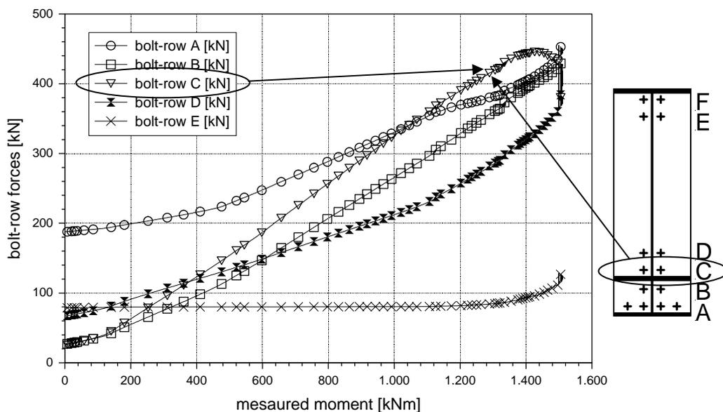
*Fig. 6.* Moment vs. bolt-row force diagrams of specimen TB3
