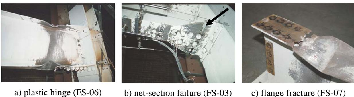
*Fig. 4.* Failure modes – Full-scale beam-to-column joints [1]
