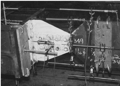
*Fig. 1.* T-stub component test [1]
