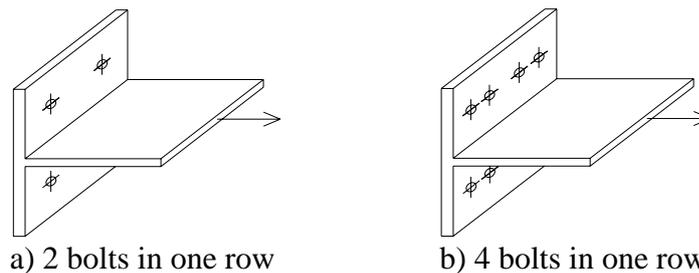
*Fig. 6.* T-stub configuration
