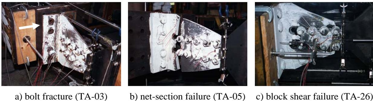
*Fig. 3.* Failure modes –T-stub component test [1]
