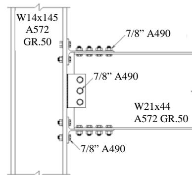
*Fig. 2.* Full beam-to column joint tests [1]
