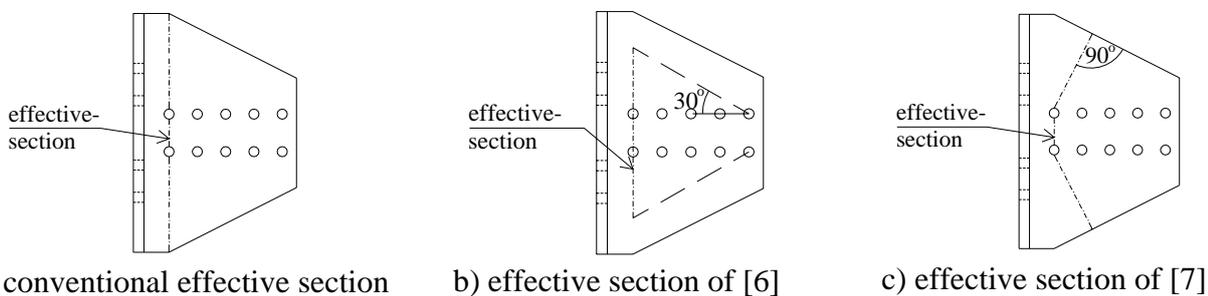
*Fig. 7.* Tapered T-stub stem
