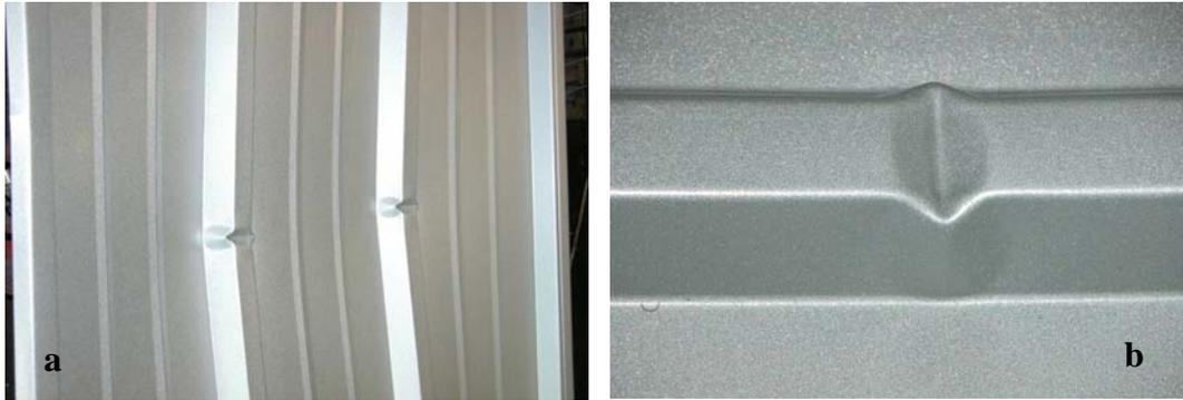
Fig. 6: Simply supported sheet failure – positive layout
