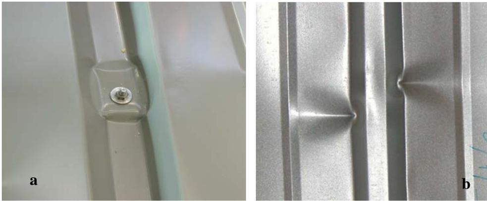
Fig. 9: Three or four supported sheet failure – negative layout
