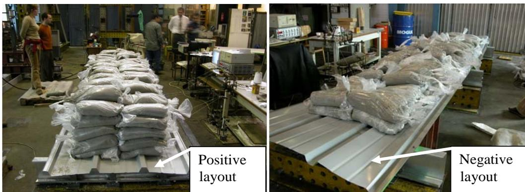
Fig 2: Test and loading arrangements
