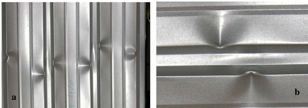
Fig. 7: Simply supported sheet failure – negative layout
